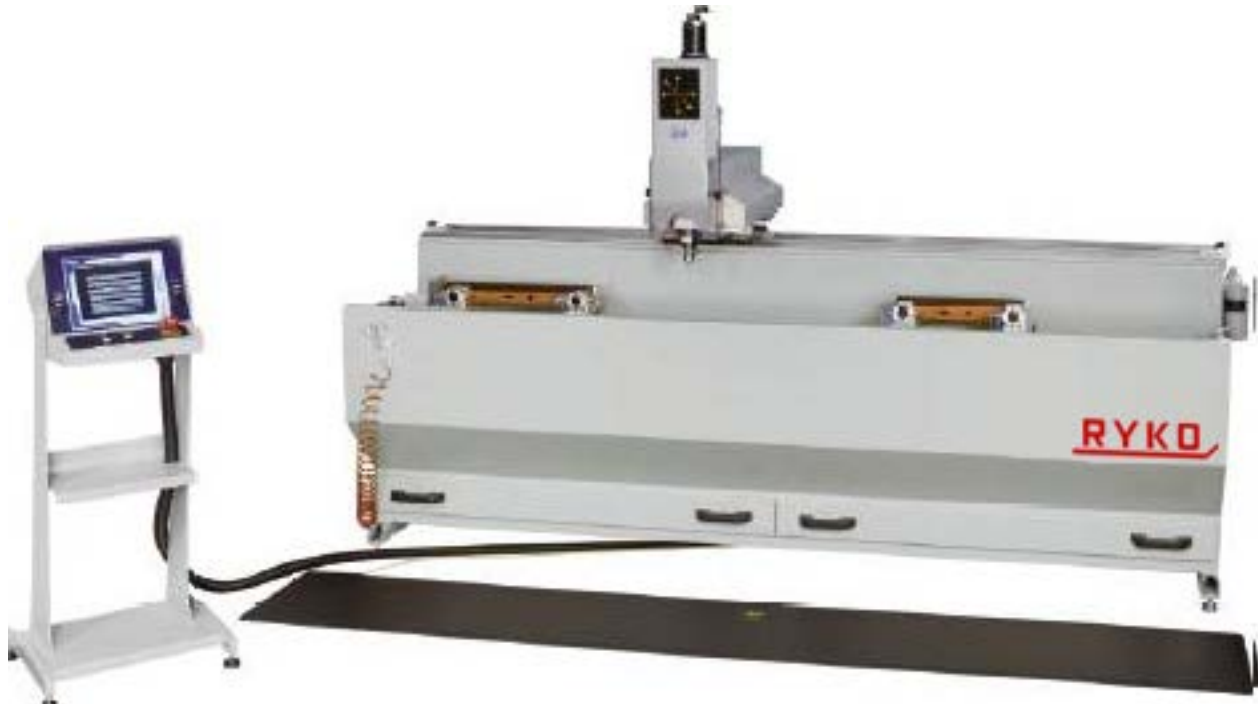
Abb.: Junior CNC – with safety carpet and light barrier
